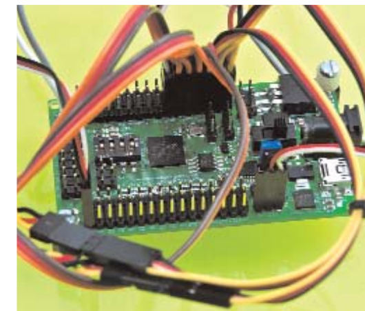
The Yost ServoCenter Mini controller board is used to control the 6 servos on the SG6-UT robotic arm as well as the power relay for the Handi-Vac suction pump. It connects to the PC using a standard USB mini cable.
