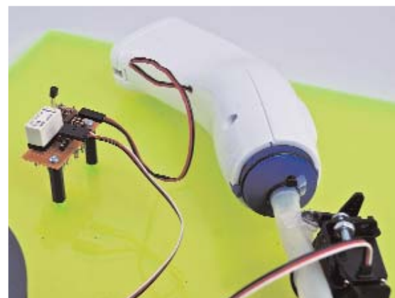
Close-up view of the servo assembly that controls the release of suction. Note the small hole in the tubing that is used to allow air to pass back into the system.
