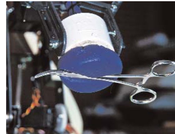
BalloonBot's grip is adaptive and strong. It has no problems picking up forceps.
