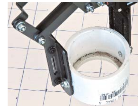
Close-up of the PVC coupling used to hold the coffee filled balloon. Note the short piece of PVC pipe at the bottom which forms a ridge that the balloon will grip when suction is applied.
