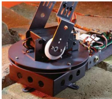
The completed SG6 arm has a sturdy pivot table to which the arm is securely mounted. In the background, the Parallax Board of Education prototyping board is visible. The “grilled” plate at the top of the arm is a sensor bracket.
