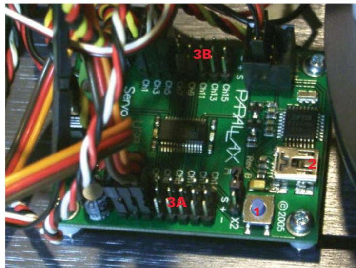
Servo Controller board. 1. Reset button; 2. USB programming connector; 3A and 3B. Servo connectors.
