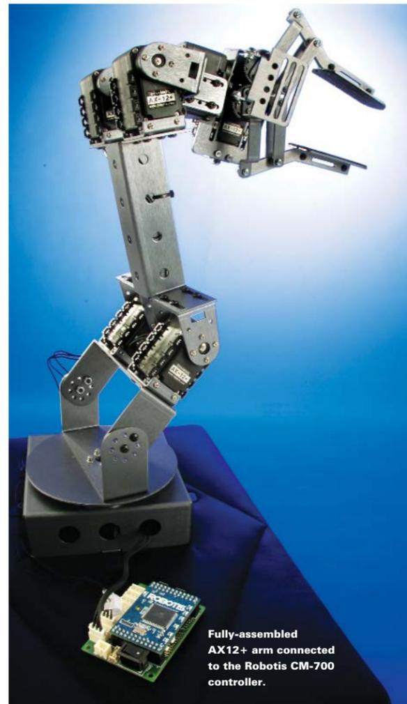
Fully-assembled AX12+ arm connected to the Robotis CM-700 controller.
