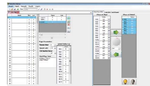
The RoboPlus Motion Editor which is used to capture positions of the arm and turn them into pose steps.
