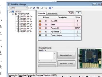
RoboPlus Manager screen showing details on the seven AX-12 servos.
