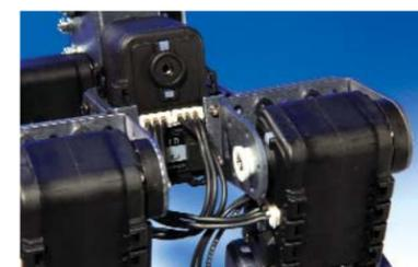
Once the arm is assembled you need to neat up the wires using tie wraps. Since the bottom of the main channel is open, it makes the perfect place to conceal the wires. It is important to ensure that the wires do not impede the range of motion for each servo.
