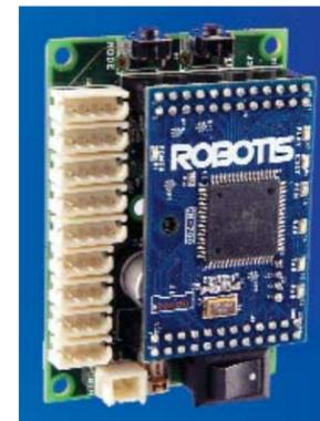
The Robotis CM-700 Controller with sub-board attached.
