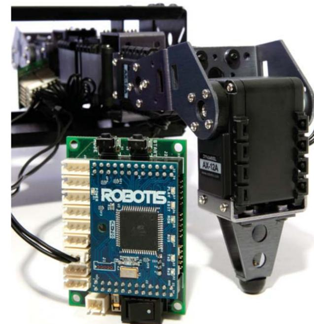
I am using the Robotis CM-700 controller to drive my AX12-18 Smart Hexapod. The controller is very robust and works well for standalone applications.
