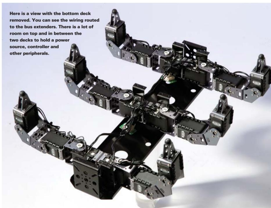
Here is a view with the bottom deck removed. You can see the wiring routed to the bus extenders. There is a lot of room on top and in between the two decks to hold a power source, controller and other peripherals.
