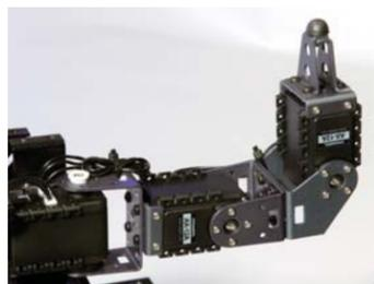
Each leg has a rubber-tipped foot that supports the robot. The rubber is a great material because it dampens the impact with the surface and provides a solid grip.
