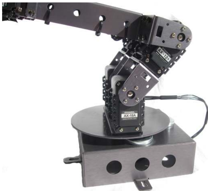
Figure 4 - 6-Axis Upgrade replaces the Adjustable Initial Angle hardware
