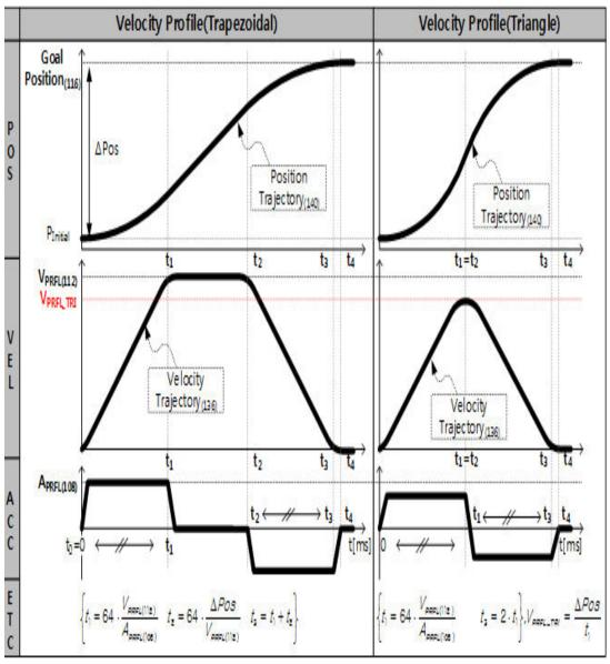
Note1): Dynamixel supports Jerk control in order to minimize dramatic change of acceleration. Therefore, actual travel time by the target trajectory of Profile could be longer than t3(t4 of above figure). Note2): Velocity Control Mode only uses Profile Acceleration(108). Step and Trapezoidal Profiles are supported. Velocity Override and Jerk control are supported as well. Acceleration time(t1) can be calculated as below equation.
