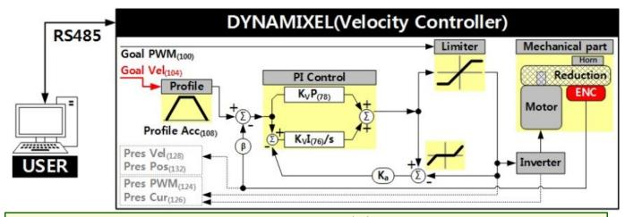
Note: K<sub>a</sub> stands for Anti-windup Gain and 'β' is a conversion coefficient of
