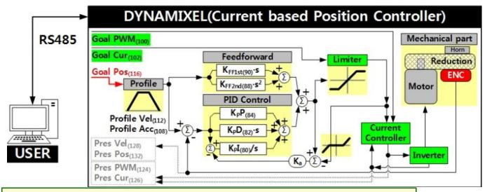
Note: Ka is an Anti-windup Gain that cannot be modified by users.
