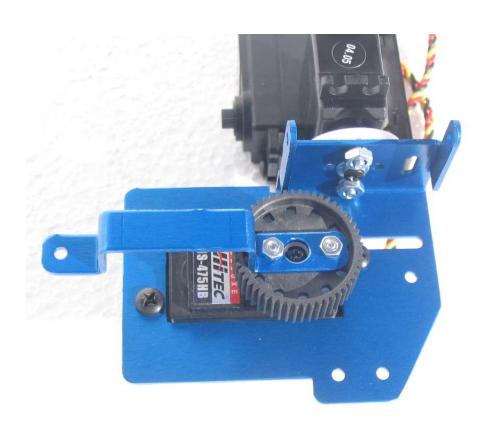
9. Using (1) 1" #4 screw, (2) washers, (1) lock nut and (1) ¼" nylon spacer, install the gear brace assembly to the palm assembly as shown in figure 11. Ensure that the gear brace assembly is aligned ("in line") with the opposite servo gear brace assembly before tightening the locknut of the assembly (see figure 12). Tighten the 1" #4 screw enough so that there is no "play" in the assembly yet loose enough to the assembly can be turned by hand.
