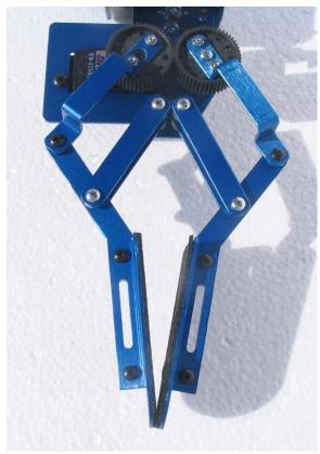
**Note:** If the gripper ends do not align when placed together, simply loosen the palm servo, slide the servo to the left to disengage the gear assembly and rotate one or both of the gear sets to align the gripper properly. Retighten the #6 screws when the grippers have been aligned.
