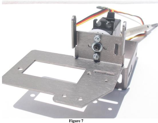
6. Using (2) #2 lock washers and nuts, install the servo arm to the pre-assembled 60-tooth gear and the servo gear brace as shown in figure 8. (Use the servo brace that has the slightly larger, offset, center hole in the middle of the 3 hole pattern). Repeat the exact assembly sequence for the opposite gear brace.
